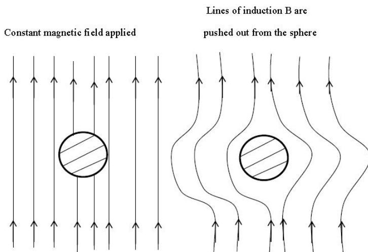
The above effect is called Meissner effect. This is due to electric currents or screening current flowing on the surface of a superconductor in such a way as to generate a field equal and
