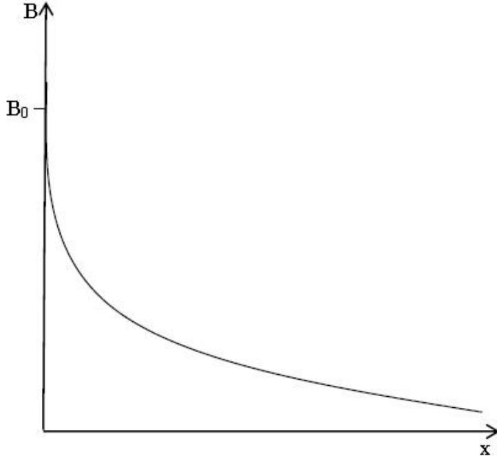
Thus the London equation predicts exponential decay of magnetic field into a superconductor occupying the region  $x > 0$ .
